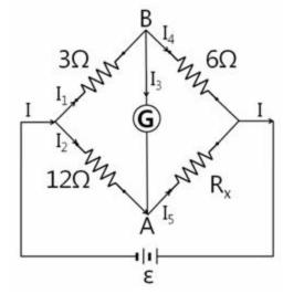
By the Kirchhoff's rule,  $I = I_1 + I_2 = I_4 + I_5$ ,  $I_1 = I_3 + I_4$ ,  $I_5 = I_2 + I_3$   $12 I_2 + 9 I_5 = -e$ ,  $3 I_1 + 6 I_4 = -e$ ,  $3 I_1 - 12 I_2 = 0$ ,  $9 I_5 - 6 I_4 = 0$   $I_3 = -0.2 A$   $I_2 = -0.2 A$ ,  $I_1 = -0.8 A$ ,  $I_4 = -0.6 A$ ,  $I_5 = -0.4 A$ e = -6 V
